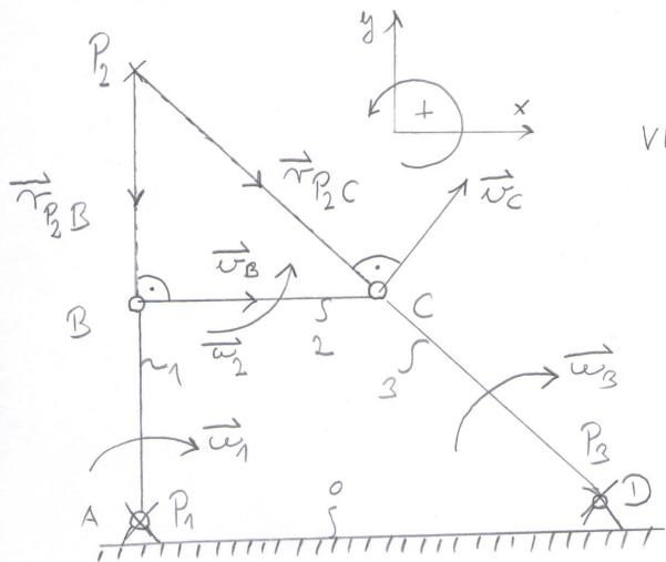
VELOCITY POLE = CENTRE POINT OF A ROTATION MOTION
