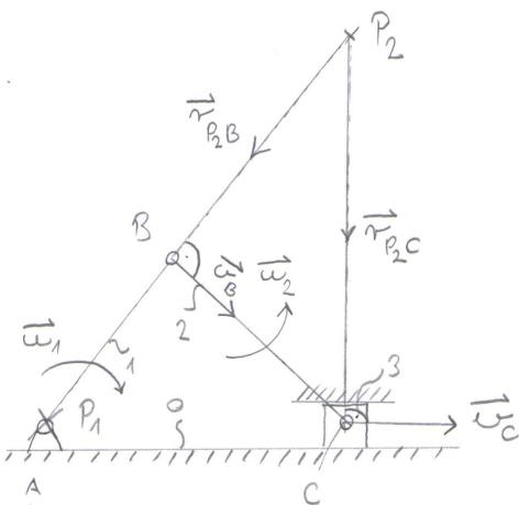
VELOCITY POLE = CENTRE POINT OF A ROTATION MOTION
