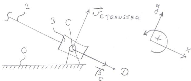
$\vec{v}_{c \text{ TRANSFER}}$ : TRANSFER VELOCITY
