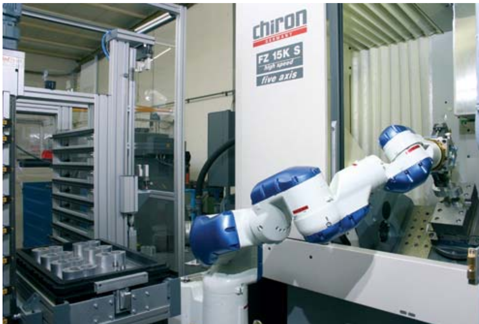
Figure 3. A 7-axis articulated robot by Motoman loading a machine center
