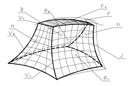
Figure 3. Surface elements and edges of hob
