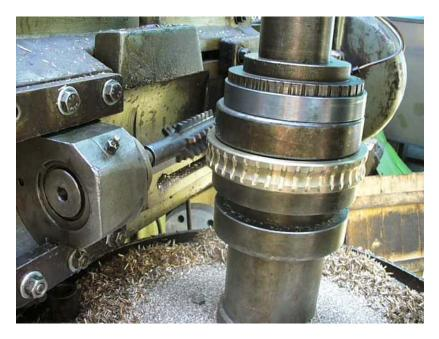
Figure 2. Worm gear production
